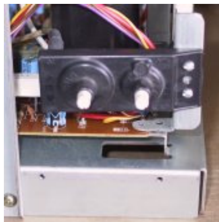
Figure 7: FA Properly Secured to Chassis
